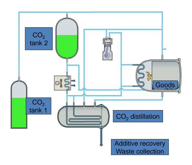
Distillation and cleaning in parallell: saves time  $\rightarrow$  short process cycle:
