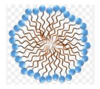
CO<sub>2</sub> Cleaning: solvent mechanism. Small molecules dissolved, heavy molecules are partly dissolved, partly "immobilized".
